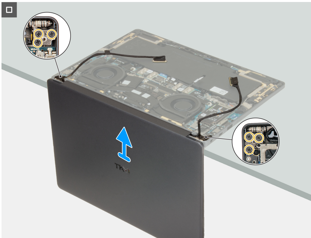
Figure 59. Removing the display assembly
