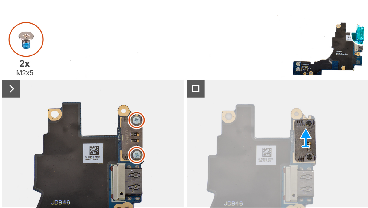
Figure 52. Removing the left USB Type-C module
